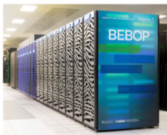
BeBop ~1,750 TFLOP/s 43,344 Intel Broadwell cores | 65,536 Intel Phi cores
