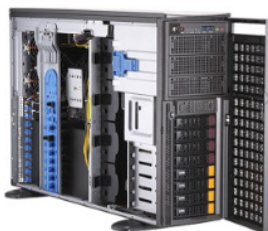
Sayre – Single node GPU system for Bragg CDI reconstructions ~111 TFLOP/s 5 x Ti 2080 | 2 x P100 | 1 x Ti 1080 | 1 x Quadro RTX 8000 GPUs
