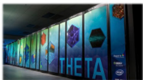
Theta & Theta GPU Theta: 281,088 Intel Phi cores (~11.3 PFLOP/s) Theta GPU: 192 NVIDIA A100s
