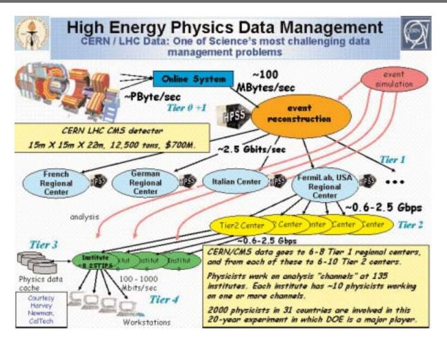
Figure A-3 A Hierarchal Data Grid as Envisioned for the Compact Muon Solenoid Collaboration. The grid features generation, storage, computing, and network facilities, together with grid tools for scheduling, management, and security.
